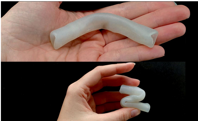
Fig. 4. The final prototype of the soft conveying toroid.
