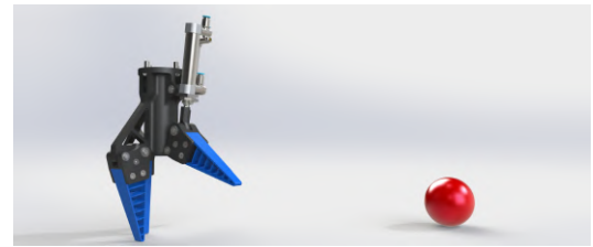
(a) Gripper in open configuration aligned with the object.
