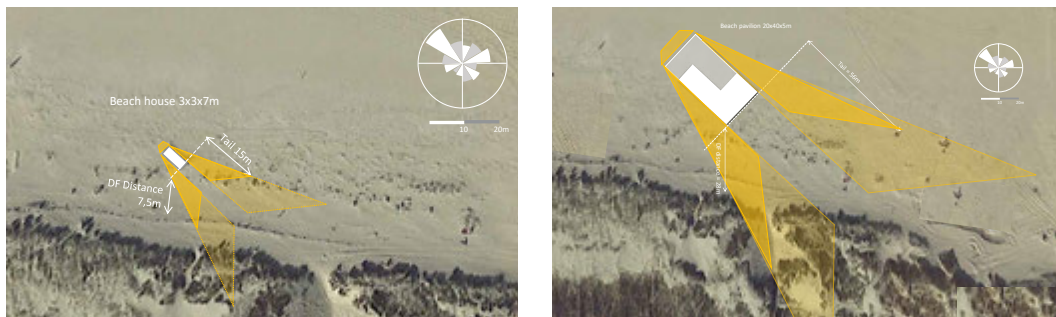
FIG. APP.A.3 Schematic sand-tail pattern of a beach house (left 3x7m, 3m high) and beach pavilion (right, 20x40m incl. terrace, 5m high). In dark yellow, the initial tails; in transparent yellow, the extended tails over time, doubling in length. Source: J. van Bergen, Aerial photo: Google earth.
