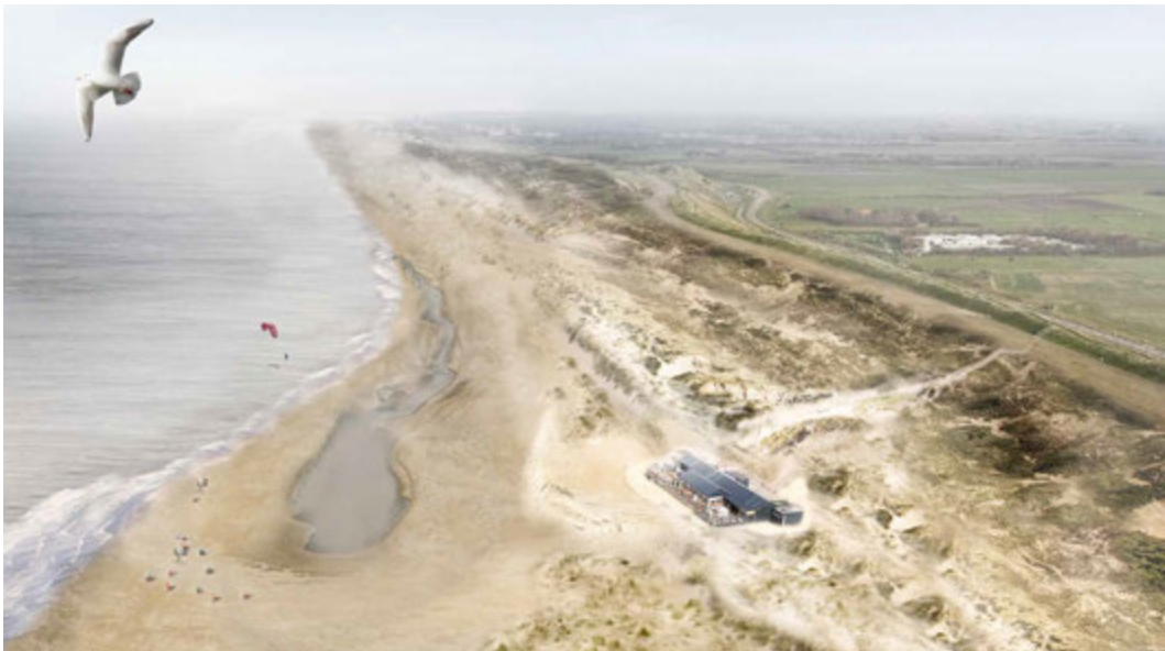
Design study phase 2: Visualisation of the progressing mega-nourishment with dune growth as coastal buffer, eco-corridor and new green waterfront.
