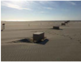
FIG. 3.59 Resulting deposition pattern around a non-elevated scale model after 6 weeks. Image by the author.
