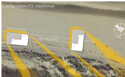
FIG. 3.68 Tail development of pavilions, elongated by their oblique setting with the wind. Source: J.v.Bergen. Aerial photo: Google Earth Pro.
