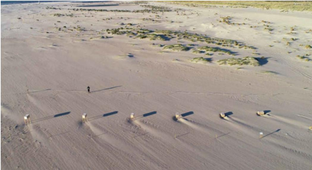
**FIG. 3.25** Final drone photograph of the deposition patterns around the scale models with increasing pole height and tail length, from 0 m (right) to 1 m (left) in steps of 25 cm. For output results, see 3.6 and 3.7. Image by the author.
