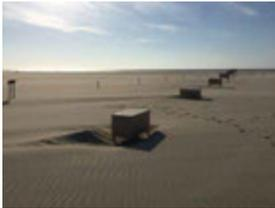
**FIG. 3.59** Resulting deposition pattern around a non-elevated scale model after 6 weeks. Image by the author.
