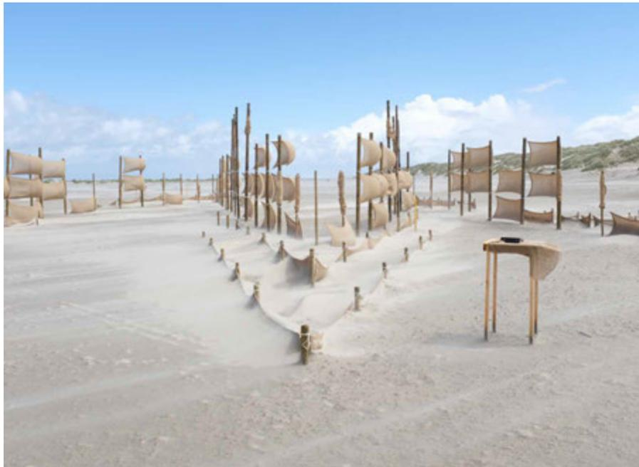
FIG. 3.55 Sediment deposition and transport around the low fences. Source: LA students TU Delft, 2018.
