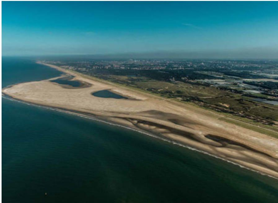
**FIG. 1.6** Aerial photo of the Sand Motor, a Dutch mega-nourishment pilot in action (2012).
