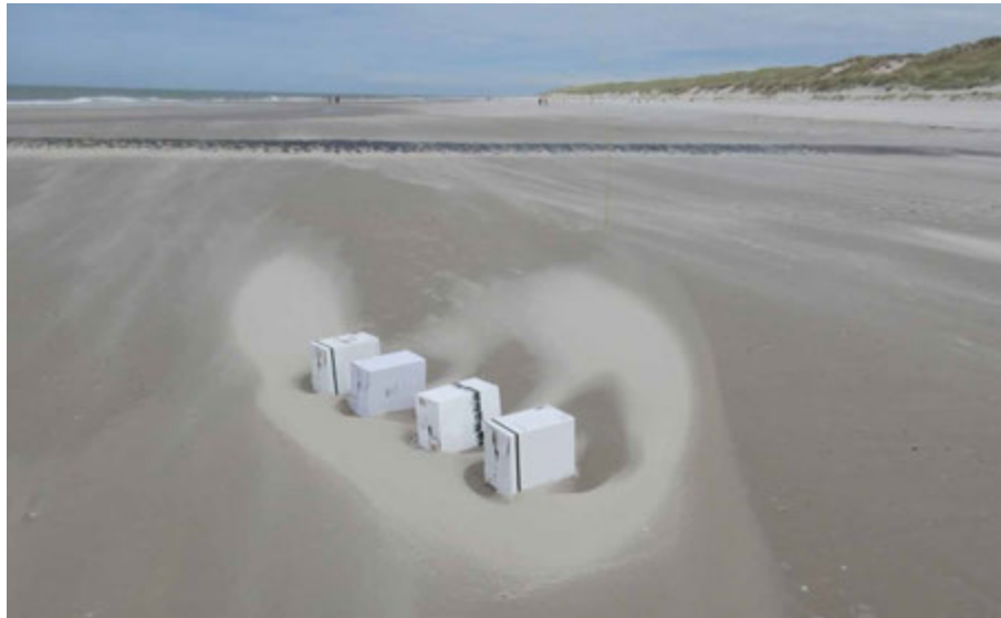
FIG. 2.32 Sedimentation pattern around a scale model of beach row housing on an angle with the dominant wind. Sand tail development can be employed to collect sediment in the foredune zone. Image by the author.
