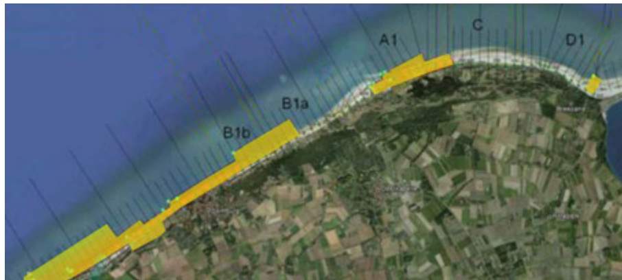
FIG. 4.16 Mapping of the 2015 nourishment programme for Walcheren, supplying sediment to maintain the coastline. Adapted from Province of Zeeland (2017).
