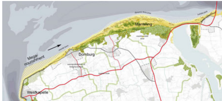
FIG. 4.18 Mega-nourishment design for west Walcheren, covering the seawall of Westkapelle with a mega-nourishment feeding the waterfront of Domburg, and leaving dynamic dune fronts to support the ecology of the Manteling in the north. Source: Studio Coastal Quality, TUD (2013).
