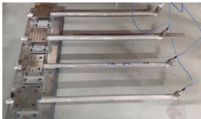
Fig. 3. Equipment for elastic modulus measurement.
