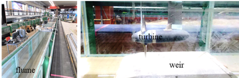
Figure 3.2: Photos from the experimental set up: a) the recirculating current flume in the Laboratory of Environmental Fluid Mechanics of Delft University of Technology, The Netherlands, b) the turbine and weir; the turbine is positioned two rotor diameters upstream of the weir end in the picture ( x/D = -2 )
