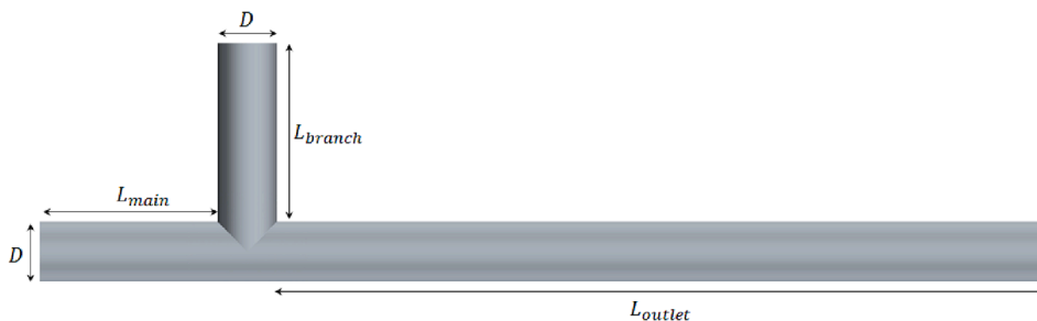
Fig. 1. T-Junction geometry employed in the present study.
