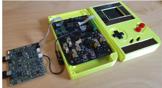
**Figure 10: DIPS connected to Engage [11] aiding in finding a memory restoration bug. After a certain time of continuous intermittent execution a checkpoint of Engage is corrupted, resulting in the handheld console failing to start.**
