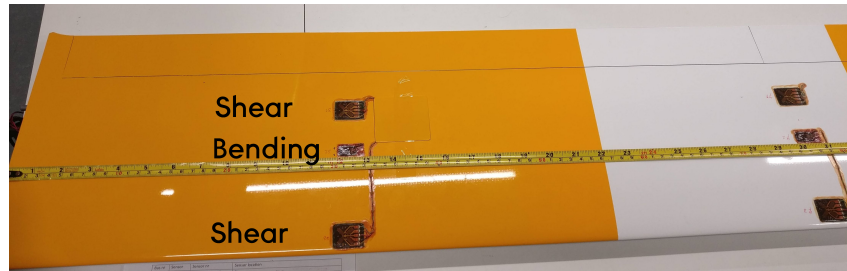
Figure 3: Strain gauge placement on the wings.
