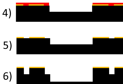
Figure 3.11: . Cross-section view of the flowchart for the silicon-based micropump and microfluidics, steps 4, 5, 6. Black: silicon, yellow: silicon oxide, red: photoresist.
