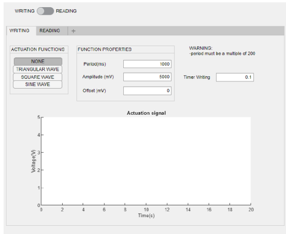
Figure 2.8: GUI developed to control the board, frequency amplitude, and shape of the actuation signal can be controlled in the writing mode. In the reading mode, the data can be saved in real-time.
