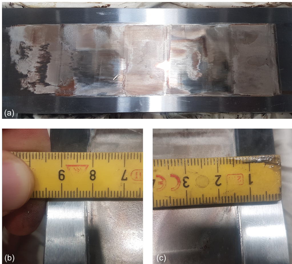
Figure 3.7: Pictures of the post-experiment inspection of the nose raceway, showing; (a) overall wear pattern comprising increased surface roughness (discolouration), pitting, and grooving, (b) close-up of grooving and surface deterioration at the lower edge in (a), and (c) close-up of grooving and surface deterioration at the upper edge in (a).
