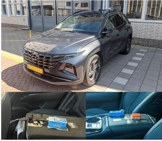
FIGURE 4. The test vehicle, a Hyundai Tucson (top), equipped with a double antenna GPS (bottom left) and IMU system (bottom right) for measuring the driving performance of human drivers.
