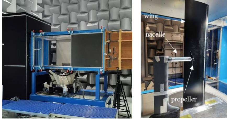
Figure 4 a) Exterior of the test section in the AWT, F15 wing model and nacelle with the propeller in the test section b). Note that one wall has been removed when taking these images.
