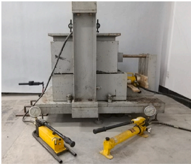
Fig. 17. Direct shear test box with dimensional sizes: 550*600*700 mm (figure reproduced from [59]).
