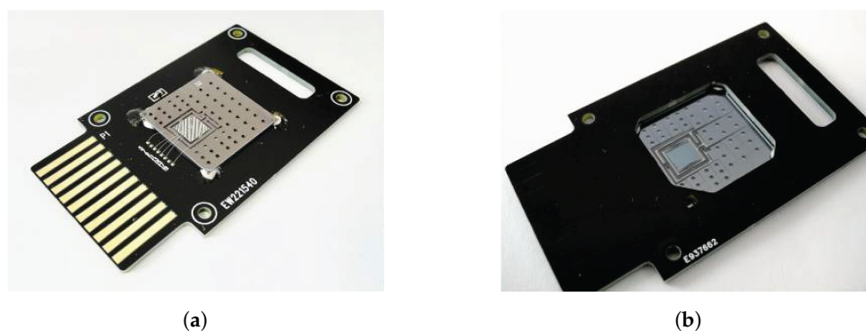
Figure 6. Microfluidic chip for DNA fingerprinting based on combination of PCR amplification and HyBeacon melting assays developed by Cornelis et al. (a) Top view of the complete chip with integrated heaters, 24 inlets, and printed circuit boards. (b) Back side of the chip showing reaction chambers and access holes connected via microfluidic channels [185] (Copyright ©2019, Cornelis et al. Published by Springer Nature. Distributed under the terms of the Creative Commons Attribution 4.0 Generic License, http://creativecommons.org/licenses/by/4.0/ (accessed on 12 May 2023).
