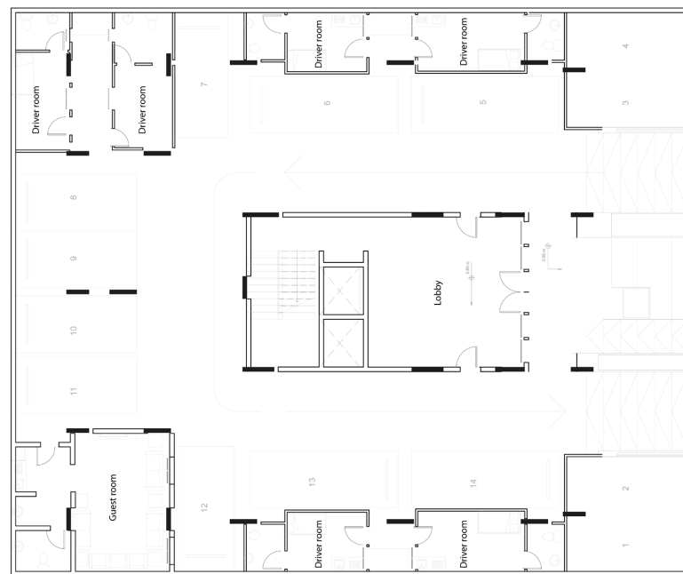
Figure 13. First floor plan (ground floor) (14 Parking spots, 6 Driver rooms, and 1 guest room).
