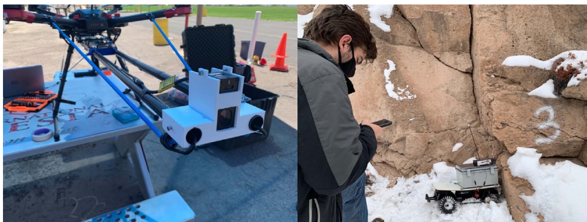
Figure 22. Robotics-based monitoring examples: (left) new aerial system of intelligent measurement integration (NASIMI) [248, 249]; (right) rock-slide detection using machine learning with BRUTUS [250, 251].
