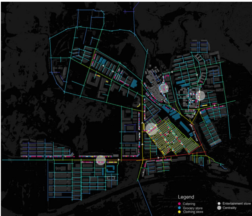
Fig. 14.7 Overlaying the mapping of retail stores and street integration analysis at R = 800 . Image Yishiqin Li, TU Delft
