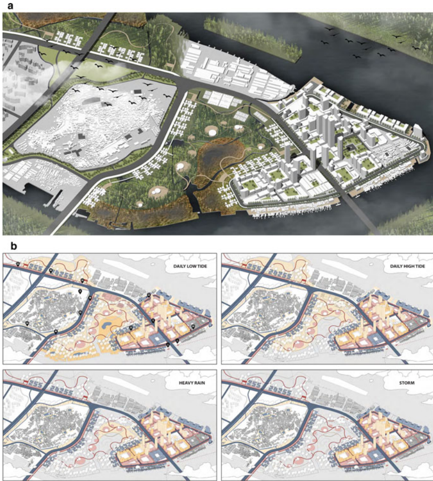
Fig. 6.3 a Bird's-eye view of the proposed masterplan for the eastern side of Pashou Island; and b diagrams showing how the site changes with changing water levels and climatic conditions. Images Jiayun Wu, TU Delft
