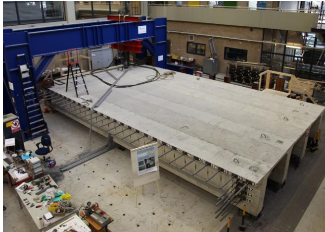
Figure 1 – 1:2 scaled model of the bridge in the laboratory
