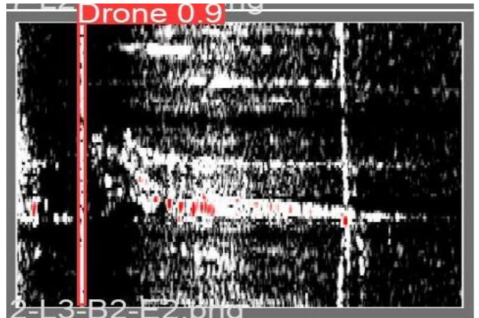
Fig. 5. Example of output of the proposed model for the same range-Doppler plot of Fig. 4, but using Adam as optimizer. The choice of this optimizer did not yield false detections.
