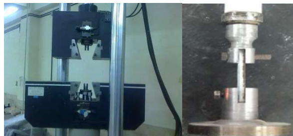
Figure 2 A DARTEC 9600 universal machine (left), The flexural tension jaw (right).
