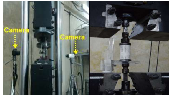
Figure 3 a) DARTEC and cameras configuration b) Dotted Travertine specimen.
