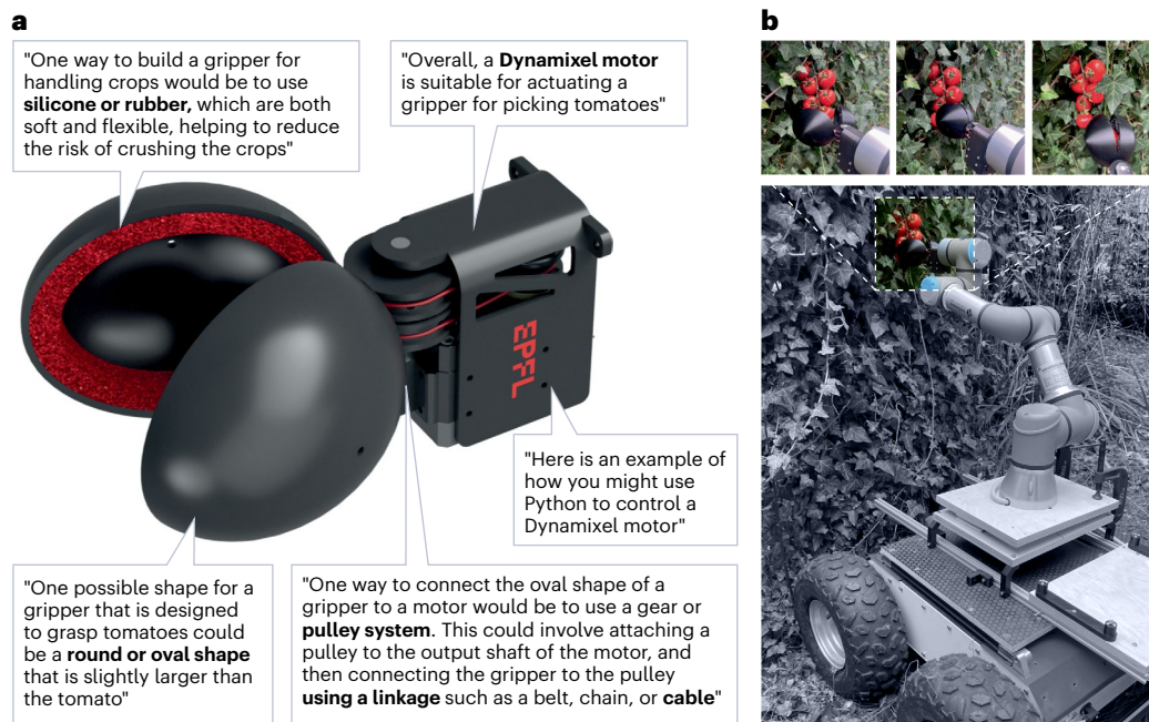
Fig. 2 | An AI model designed this robotic gripper. a , Some of the technical suggestions generated by the LLM, including shape indications, code, component and material selection, and mechanism design. b , Guided by these inputs, a gripper was built and tested on real-world tasks, such as tomato picking, as shown at right.
