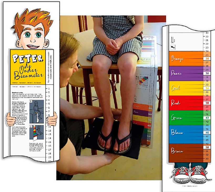
Figure 3. Measuring tool for finding fit between individual child anthropometrics and chair size mark.
