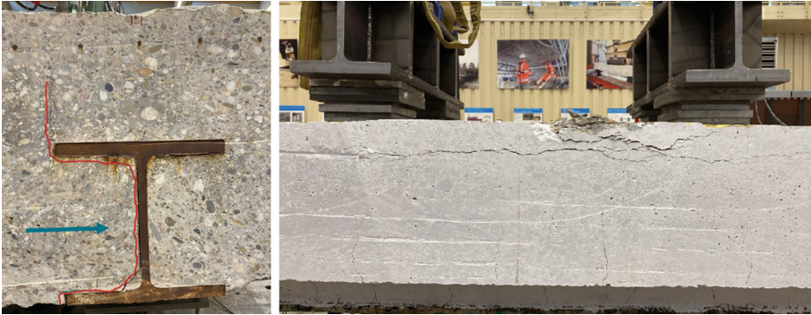
Fig. 7. Observed Failures. Left: Specimen LB1. Right: Specimen LB3
