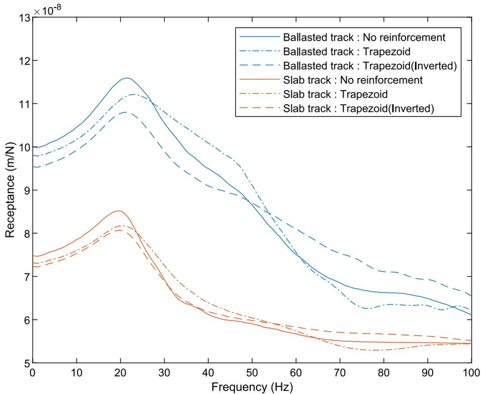
Fig. 14. Rail receptance for different earthwork configurations.
