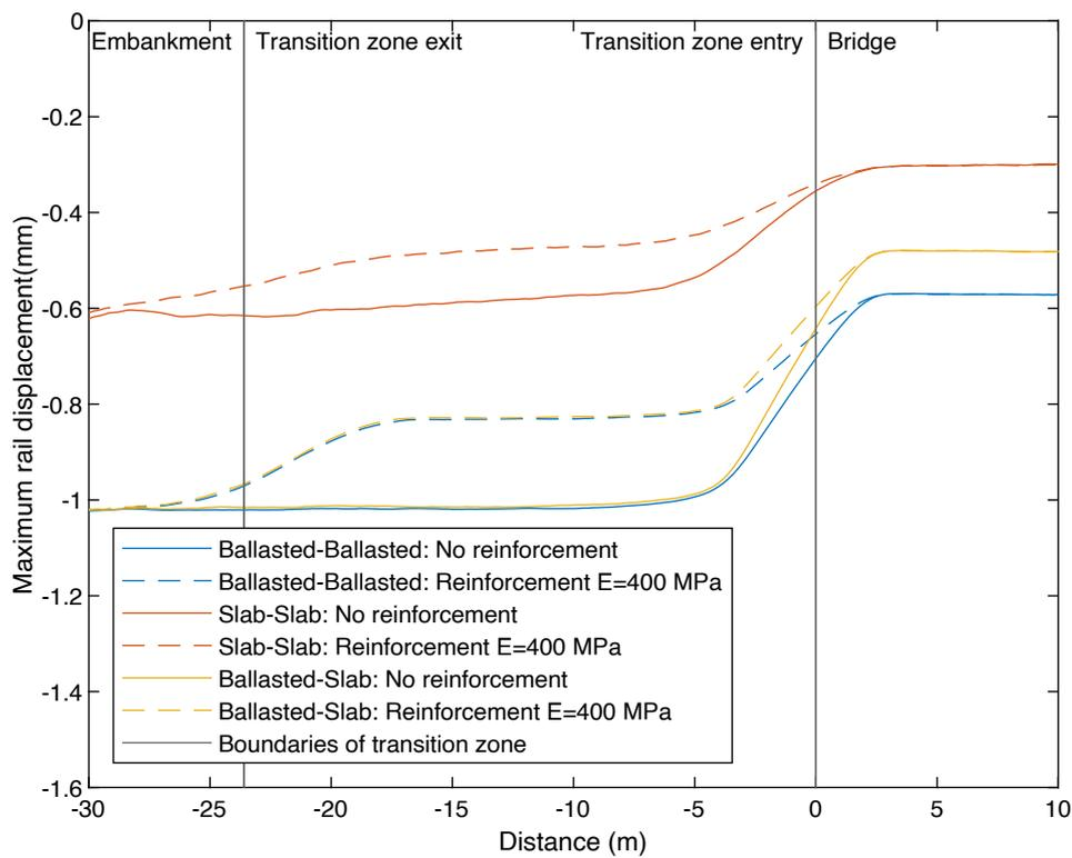
Fig. 12. Rail displacement for different track permutations.
