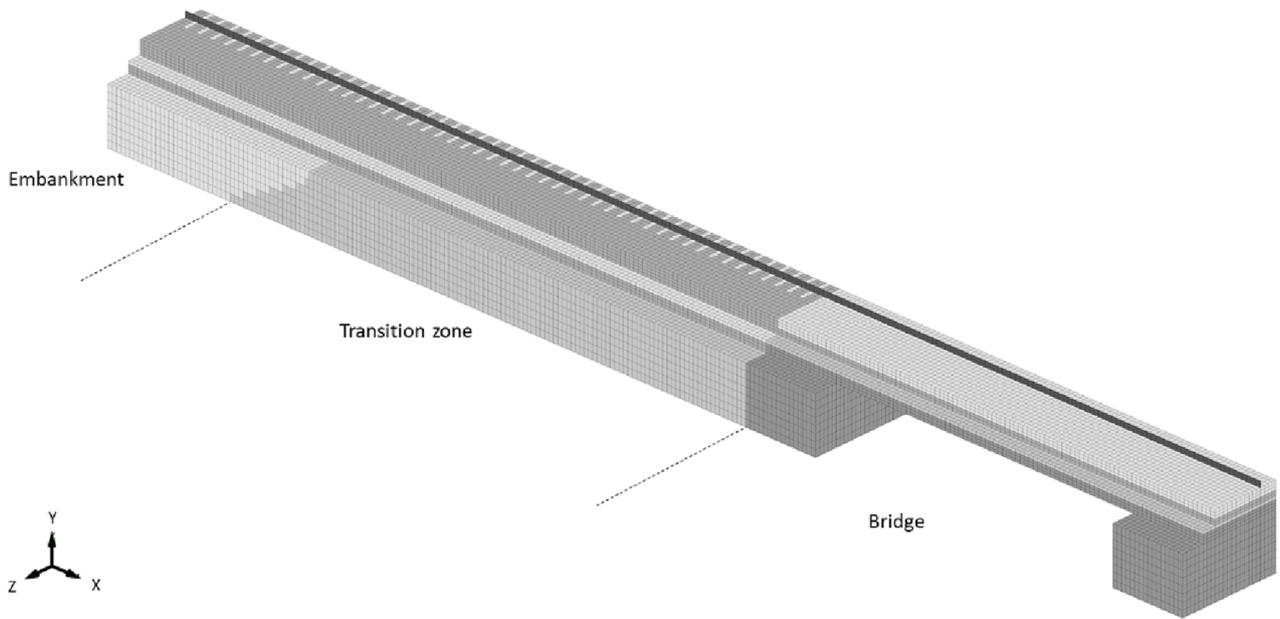
Fig. 4. Numerical modelling domain (embankment length truncated for viewability).
