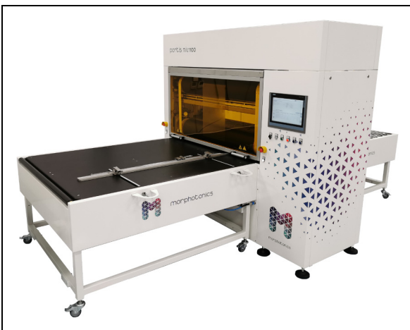
Figure 4. Morphotonics Portis NIL1100 roll-to-plate nanoimprint equipment. 41
