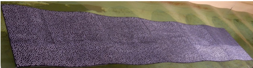
Fig. 5 Model structure with speckle pattern in the towing tank. Wave propagating from right to left
