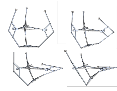
Fig. 8. CAD model of the current manipulator transitioning from translation mode to mixed freedom mode. As the center moves away from the center's vertical axis the tilt angle increases.
