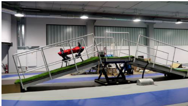
FIGURE 4. ANYmal C robot performing a benchmarking test on the EUROBENCH facility.
