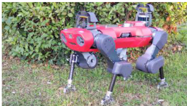
FIGURE 1. The quadruped robot ANYmal C equipped with the adaptive feet SoftFoot-Q performing a habitat monitoring mission.
