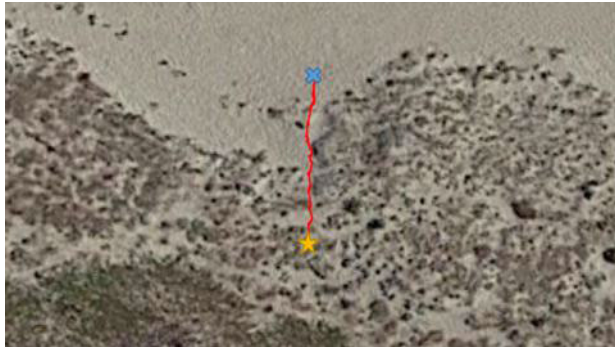
FIGURE 11. Map of the robot motion while performing the habitat monitoring mission in embryonic and white dunes. The blue cross indicates the starting point, while the yellow star indicates the final point.
