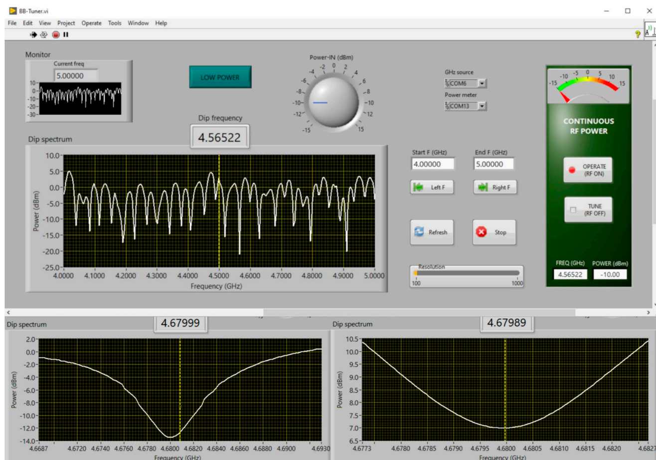
Figure 7. Screen shot of the dip-tuning program. The LabVIEW program monitors the signal from the power meter as a function of the scanned microwave frequency. ( Upper panel ) After an initial choice of frequency limits (here: 4–5 GHz), the program produces the power response at -10 dBm input power. A cursor is then used to single out an individual dip, using the 'left' and 'right' buttons; ( lower left panel ) this dip peak is re-scanned at low power and is then further reduced, using the cursor, to limiting power levels of circa 4 dB above the dip power; ( lower right panel ) input power is raised such that a dip power ensues that will be optimal for the detection diode, that is, circa 0–10 dBm. The bridge is now tuned and can be turned to permanent RF output ('operate'), and reflected power can be switched, with the SPDT switch, to the detection diode for EPR spectroscopy.
