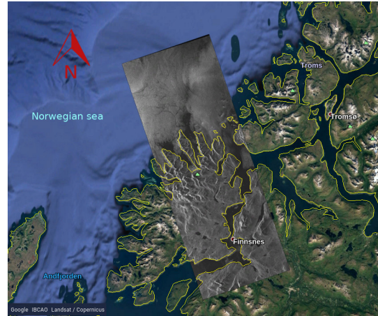
Fig. 4. BiDi ATI acquisition at the coast near Tromsø. The latitudes of the image vary between 68.9°N and 70.3°N and the longitudes of the image vary between 17.7°E and 18.6°E. The width of the strip is 30 km.
