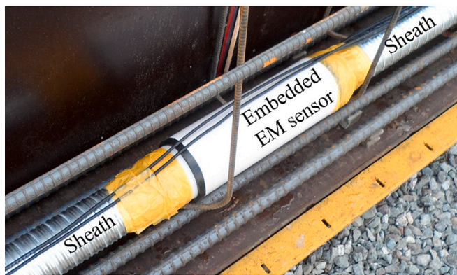
Fig. 18. Embedded EM sensor and its sheath on carbon steel tendon as core (taken from [54]).
