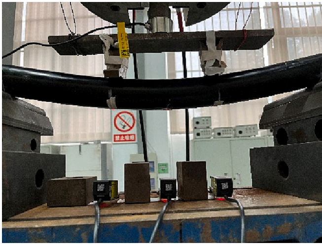
Fig. 18. Bending illustration of a cable sample.
