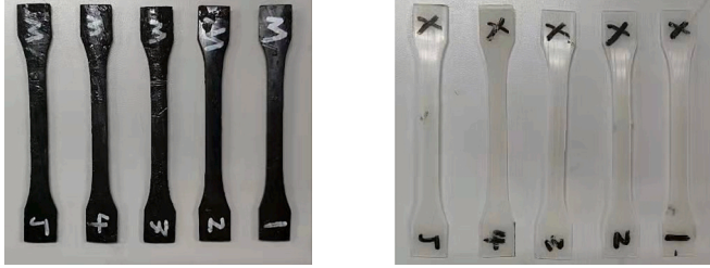
Fig. 11. Dumbbell shape of MDPE (left) & XLPE (right).
