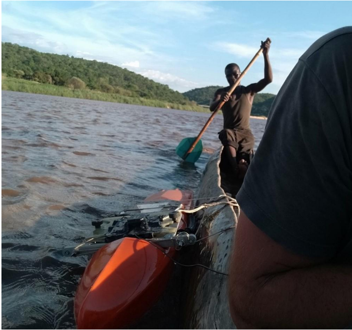
Fig. A1. ADCP with a Low-cost RTK GNSS attached to canoe
