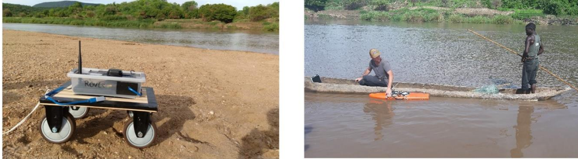
Figure 5.4 (a) Low-cost RTK GNSS rover mounted on a mobile cart for recording RTK waterline 5 and (b) ADCP combined with an RTK
