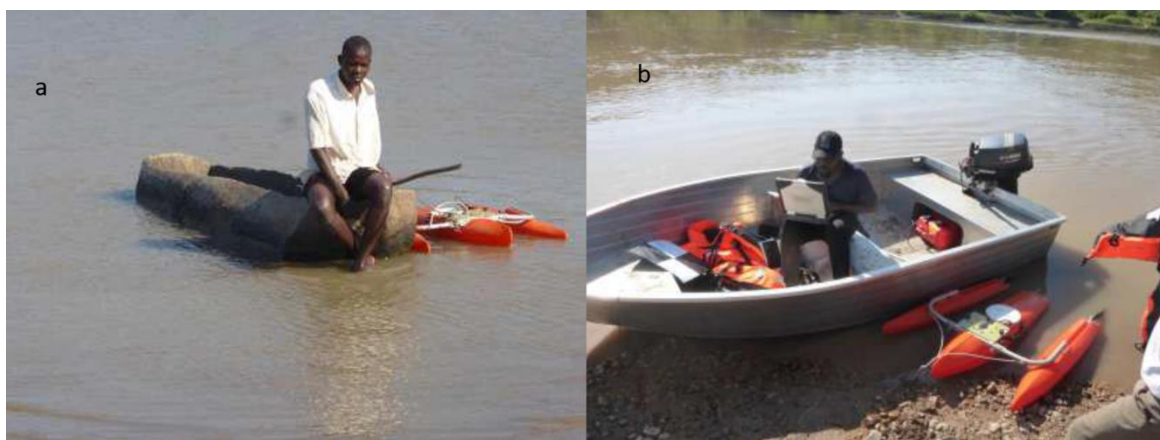
Figure 3.1 a) ADCP attached to Canoe b) ADCP attached to motorised boat (Section 5.2.6 presents the method by which the ADCP was used)
