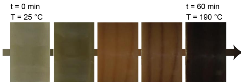
Figure S3 Photographs (projected sideways) of the COF reaction mixture in the Taylor-Couette reactor with increasing reaction time and reaction temperature from left to right.
