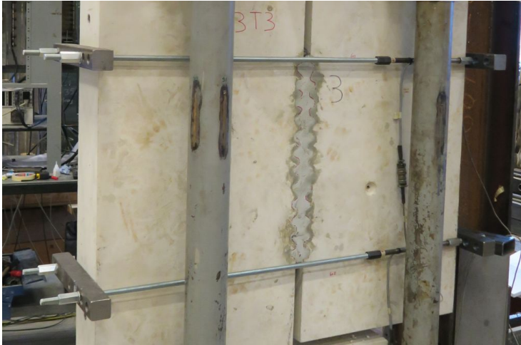
Figure 5.25: Lateral stiffness provided by steel bars, transverse blocks and precast concrete L-elements
