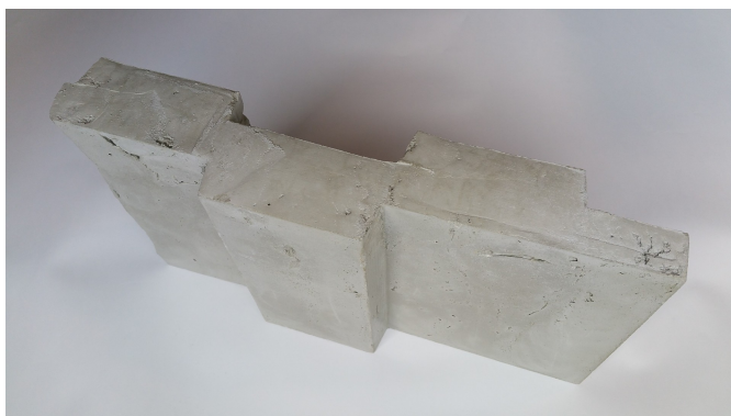
Figure 4.3: The mortar filling after demoulding
