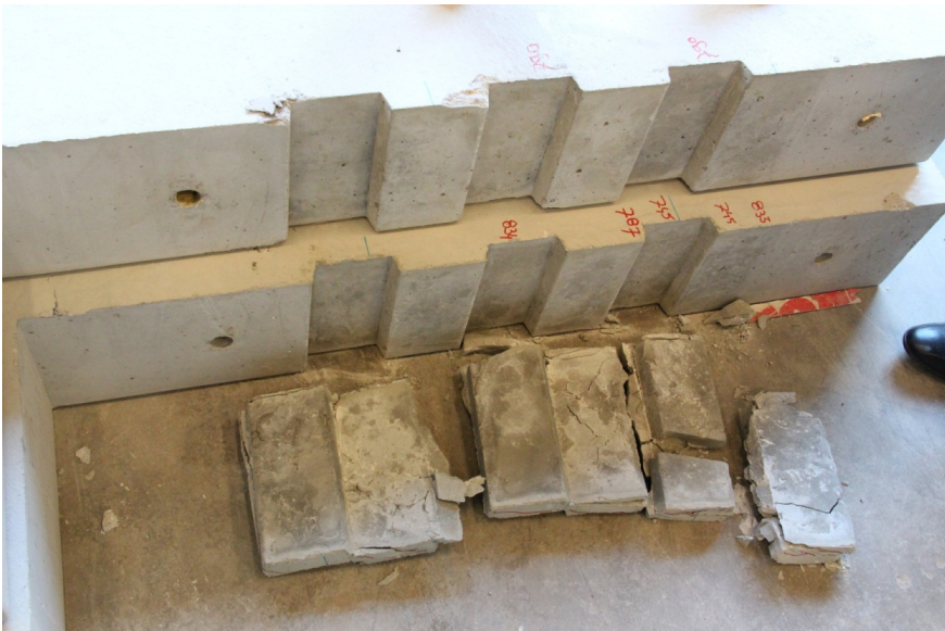
Figure E.5: Specimen 2-7: Dismantled specimen (Tiksomortar K70)
