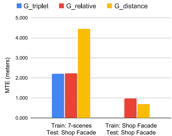
Fig. 7. MTE of the three encoders used for testing VPR-based localization on the Synthetic Shop Facade dataset, when trained on the same and different dataset. Notably, G_{\text{triplet}} and G_{\text{relative}} trained on the 7-scenes can outperform G_{\text{distance}} trained on the 7-scenes dataset. However, G_{\text{distance}} when trained and tested on the Synthetic Shop Facade dataset performs the best. Since the Shop Facade dataset contains images of only one scene, unlike the 7-scenes dataset, we could not select proper negative images in this dataset and do not train G_{\text{triplet}} on this dataset.
