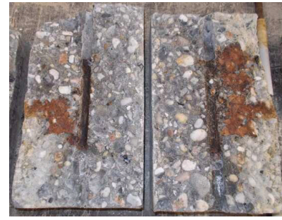
Fig. 8. Picture of a split sample after a pull-out test.
