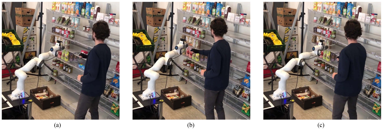
Fig. 5. DF in the presence of a human. The human hand's state is estimated with a motion capture system. The robot smoothly and in advance avoids the human operator and allows for safe coexistence. (a) t = 0 s. (b) t = 2 s. (c) t = 3 s.
