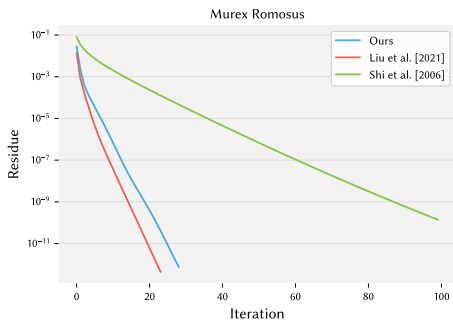
Figure 9: Residual over iteration count for Ours, Liu et al. [2021], and Shi et al. [2006] for data smoothing on Murex Romosus with \alpha = 1 \times 10^{-3} . See Figure 1 for a plot over time.
