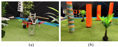
Fig. 7. (a): Experiment platform for real world tests. (b): High-precision point cloud map built by a lidar sensor.
