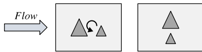
Fig. 1. Example of two rough surfaces with identical roughness elements and averaged local quantities, such as their skewness or their kurtosis, but different hydrodynamic behavior (Forooghi et al., 2018).
