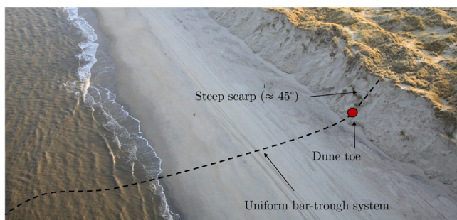
Fig. 2. Dune erosion at the coast of Vlieland, the Netherlands. Photograph by van Houdt (Dutch Ministry of Infrastructure and Water Management) (2008).
