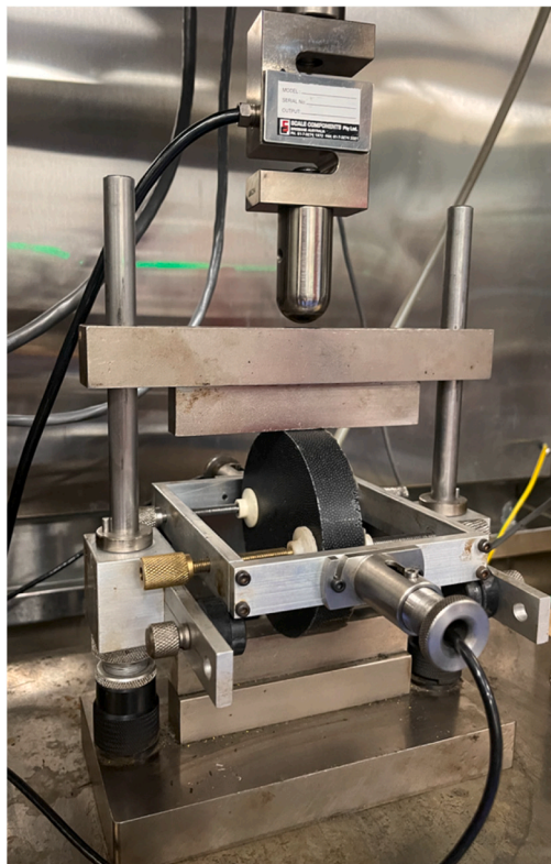
Fig. 8. Setup of indirect tensile stiffness modulus test.
