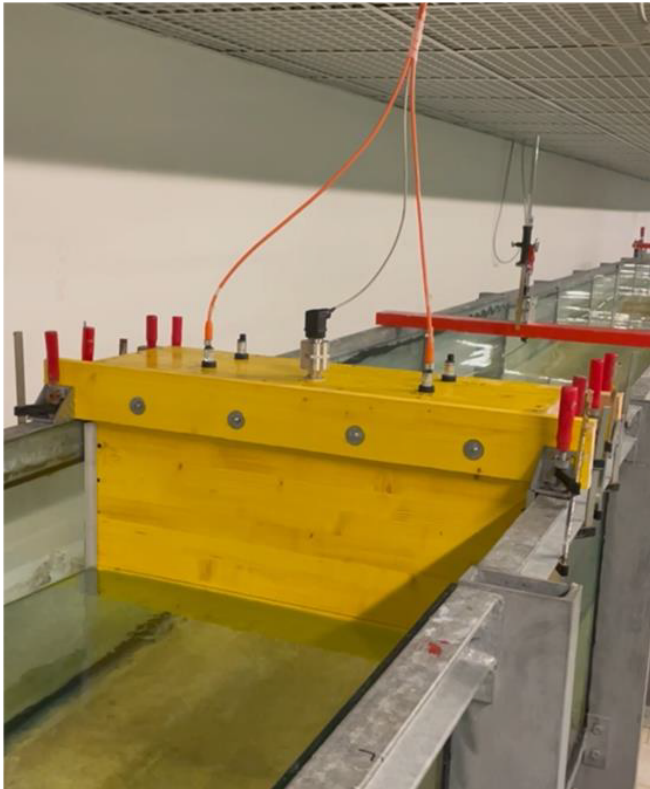
Fig. 4. BOX OWC placed in tank - WG4 and WG5 are wave gauge designated by orange wires and PT is the pressure gauge depicted by the black wire
