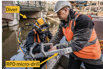
Fig. 10. RPD deployment underwater by a diver.
