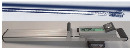
Fig. 11. Microdrill (upper picture), drilling device below.
