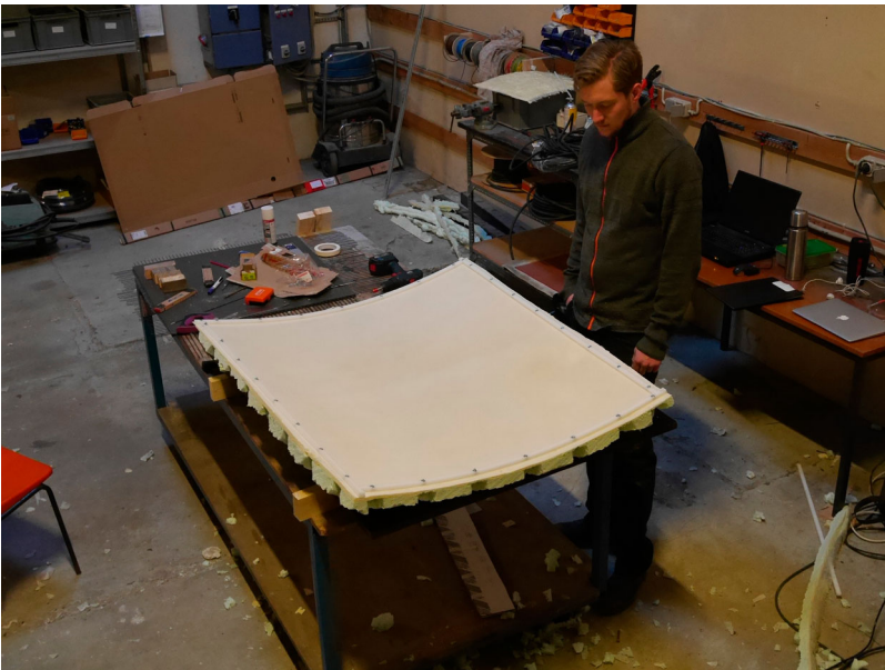
Figure 29. Finished intermediate mould ready for being tested with sprayed GFRG.
