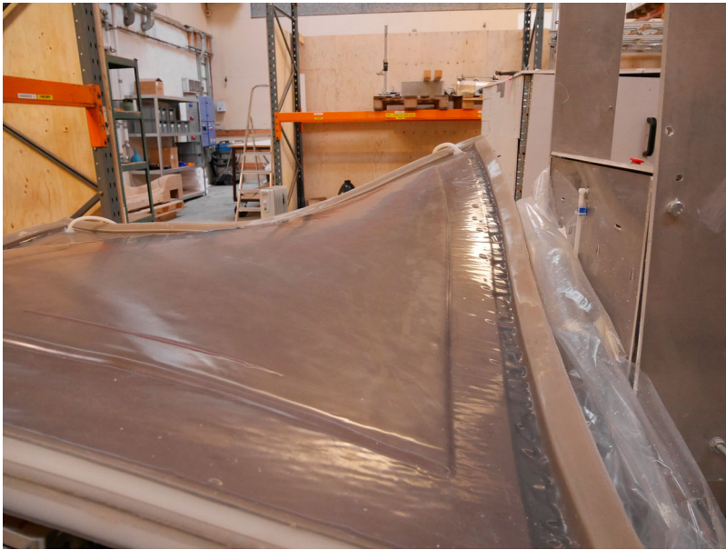
Figure 19. Setting out of the tested mould shape on the flexible table.
