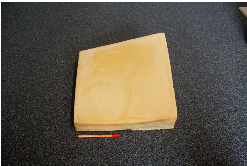
Figure 9. First sample of intermediate mould made with LDPU ( 40 \times 40 \text{ cm} ).
