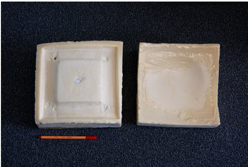
Figure 13. Small scale (23 × 23 cm) sample two-part intermediate mould for use with the premixed method.
