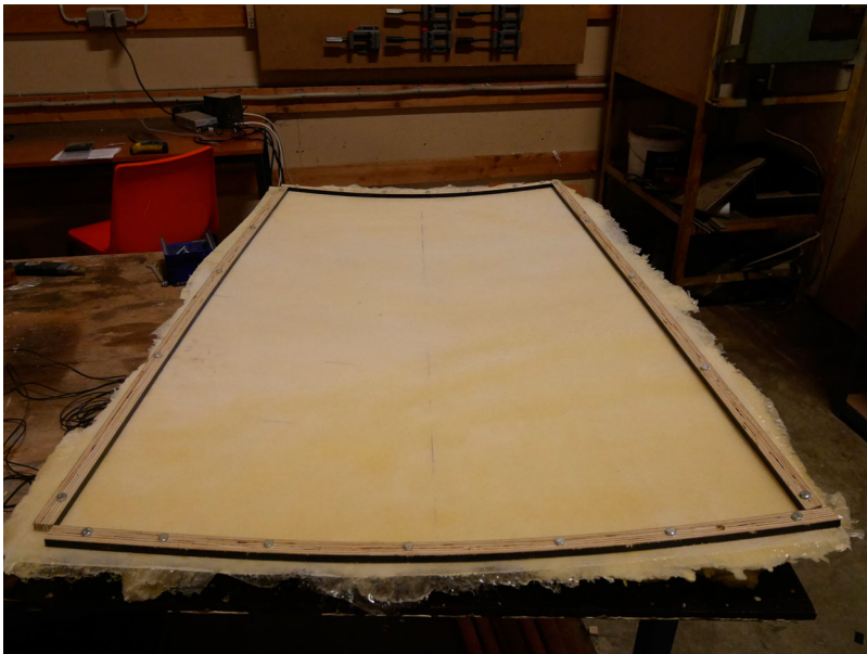
Figure 18. Fitting timber edges barriers on the mould.
