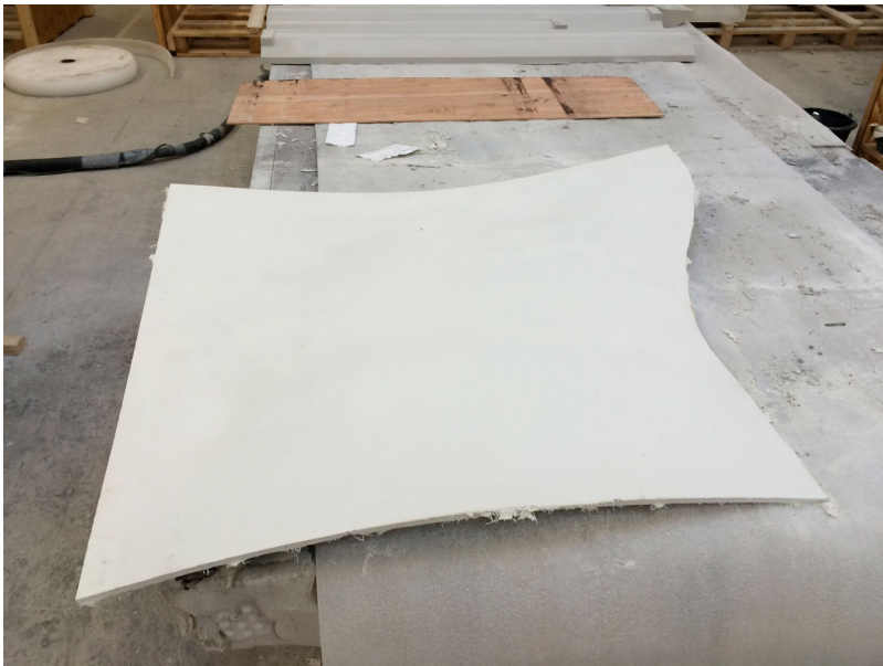
Figure 25. The finished free-form GFRC panel after demoulding.
