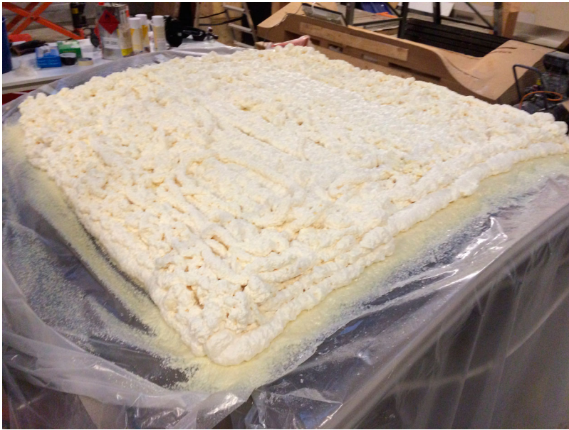
Figure 17. Curing the LDPU on the flexible table.
