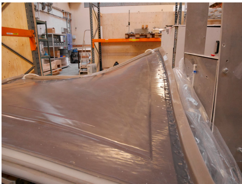
Figure 19. Setting out of the tested mould shape on the flexible table.
