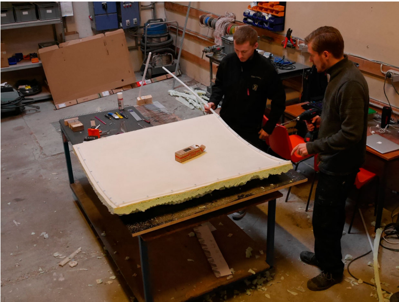
Figure 28. Plastic edge-barrier being fitted to the intermediate mould.
