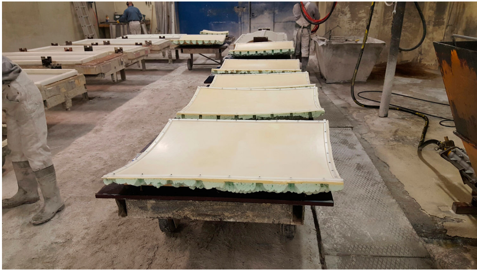
Figure 35. Intermediate mould for ring 3–9 of the thin-walled GFRC hyperbolic shell before the first casting.
