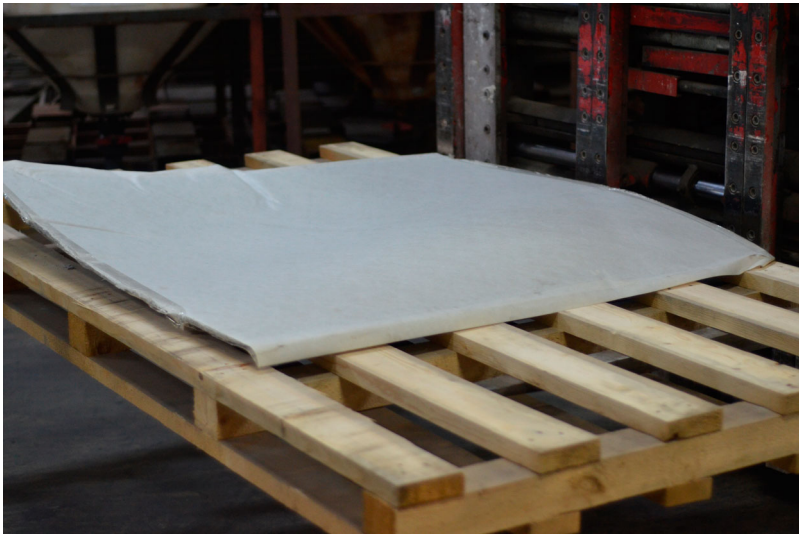
Figure 8. The automated premixed GFRP panel after curing and removal of protective foil. Panel 1,2 × 1,2 m.
