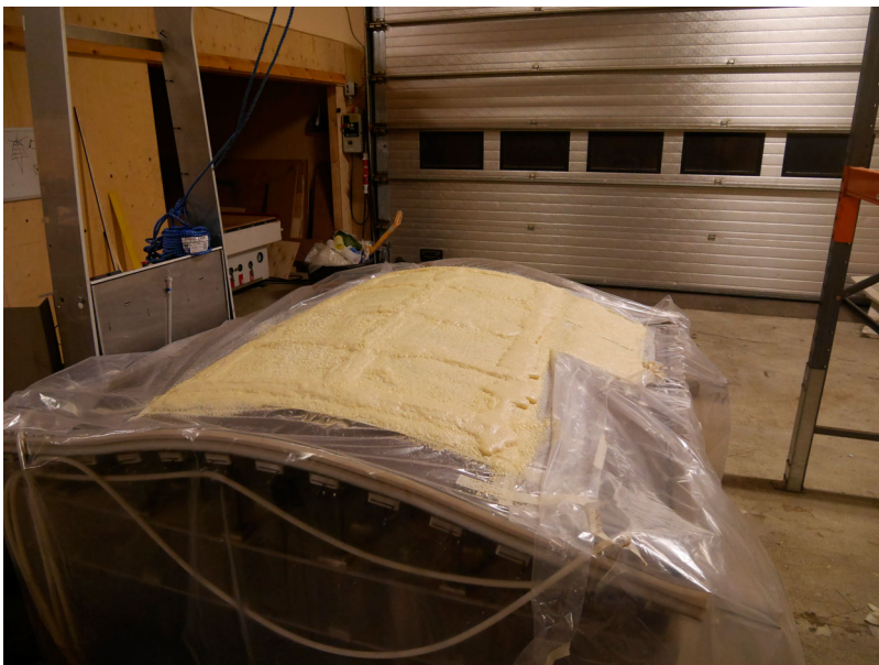
Figure 16. Curing of the HDPU foam on the flexible table.
