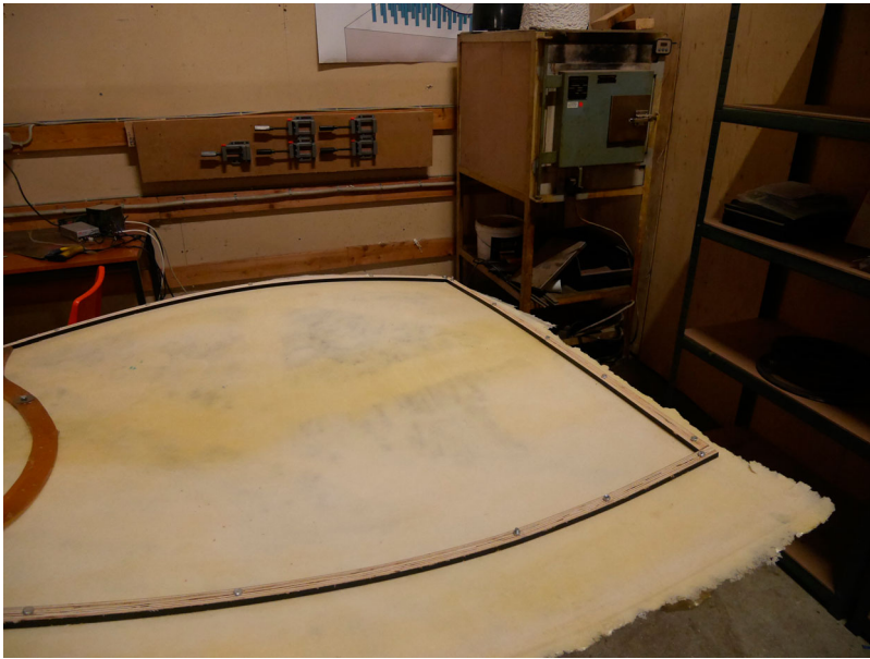
Figure 22. Fitting edges on the mould.
