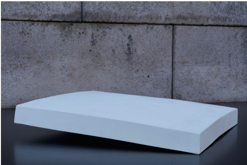
Figure 31. Finished double curved panel with a 40 mm edge-return.
