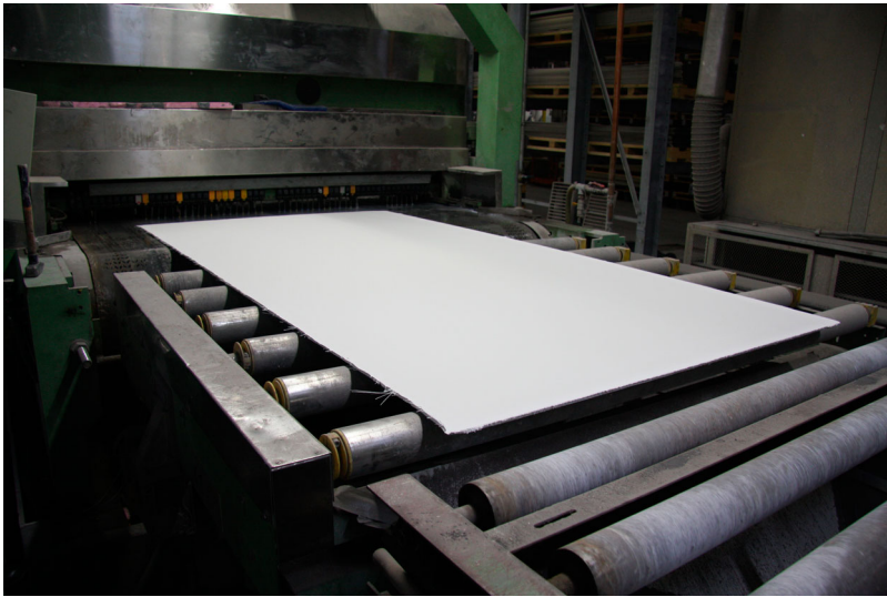
Figure 6. Automated production process for flat thin-walled GFRP (shown panel size ca 4 \times 1.2 m).
