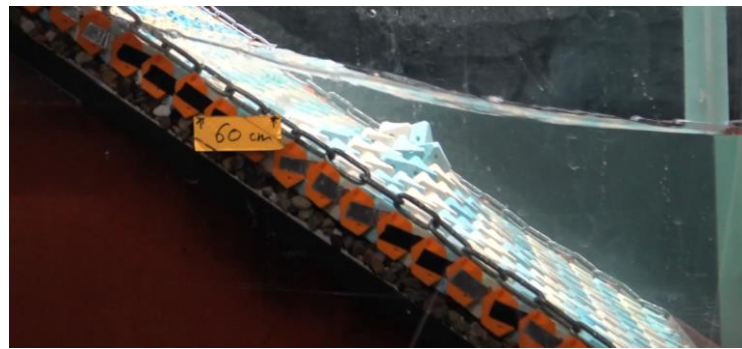
Figure 10. Effect of breathing on the armour (Molenkamp 2022)
