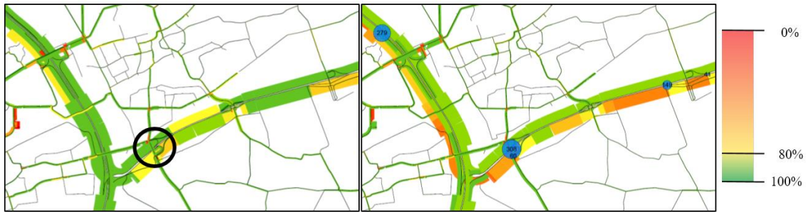
Figure 3.10: assignment results for reference scenario; static (left, black circle indicates bottleneck location) vs STAQ (right). Bandwidth colours: modelled speed as ratio of free flow speed; Bandwidth widths: modelled flow; Blue circles in STAQ results (right): vertical queues (radius indicates queue size)
