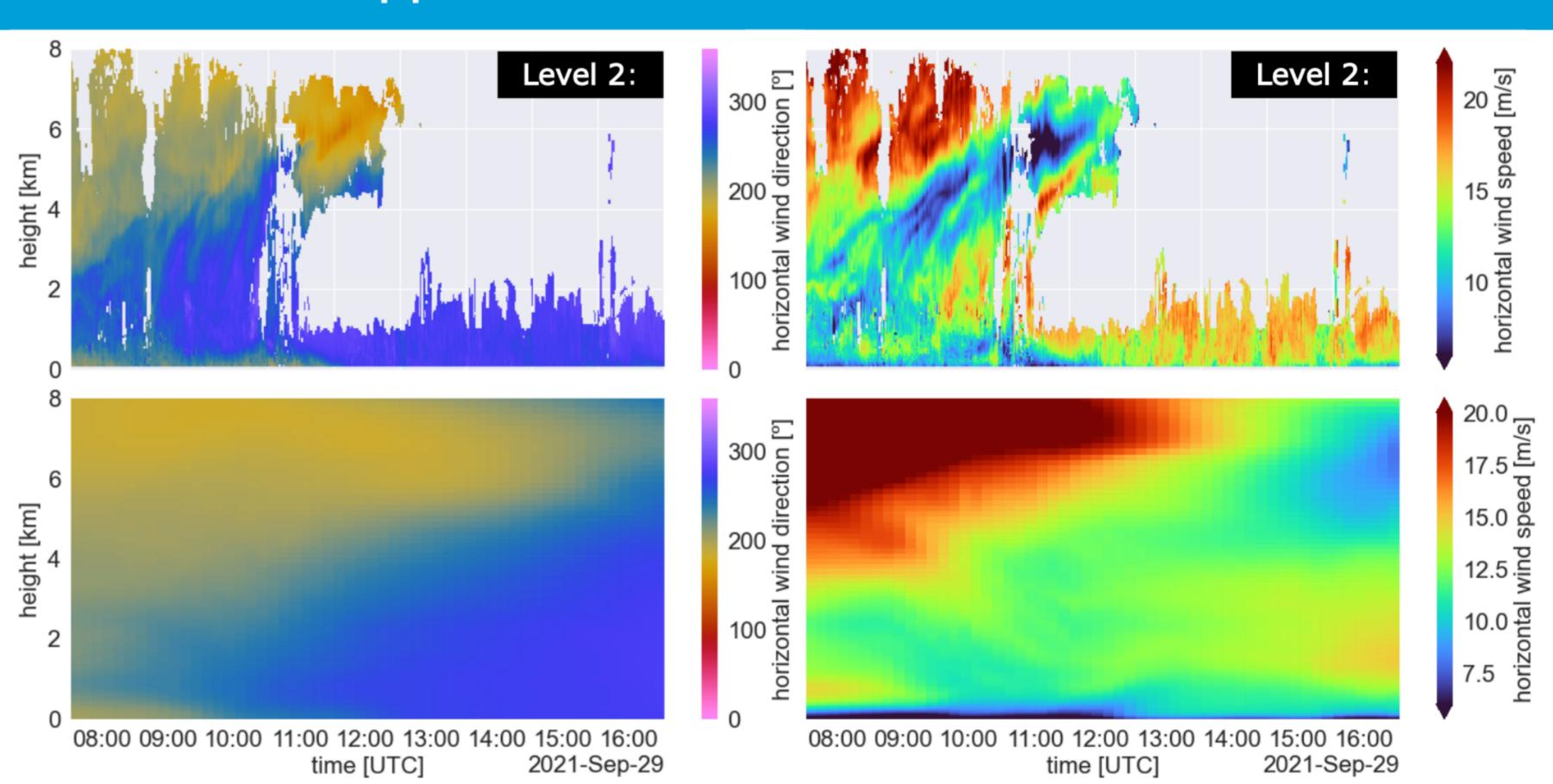
The observations and DALES' simulation show similarities in large-scale processes. For example, the change in direction and speed between 7 and 12 UTC.
