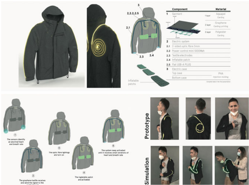
Fig. 18 Visualizations and prototype of JACKTIVE: a sportive jacket to alert for panic attacks. Project by Diego Piracoca, Sara Kashfi, Sonia González and Bianca Muresan
